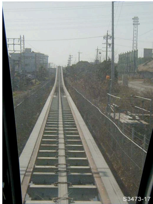
Figure 3-14. Vertical Curve at CHSST Test Track
