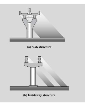
Fig. 3—Slab versus Guideway Cross-sections. The guideway structure lets through a lot more light than the solid slab, and the simpler structure of the guideway is aesthetically less obtrusive and harmonizes better with urban environments.
