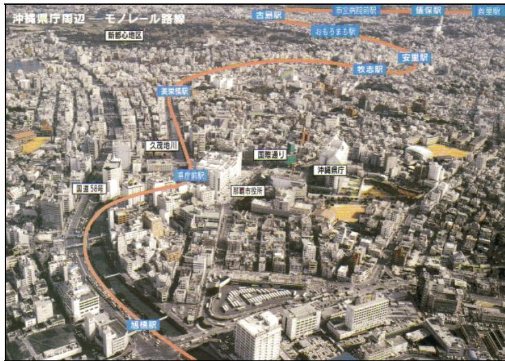
Figure 2.2—Alignment of the Okinawa system through Naha city. Tight turning radii and a narrow crosshead profile mean that straddle monorails can be fitted into dense urban alignments. Source: Yui Rail
