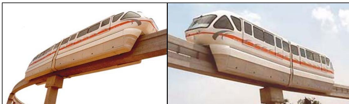
Figure 2.17—Monorail Malaysia two-car monorail train. Monorail Malaysia trains can be semi-permanently coupled into trains as long as twelve cars. Source: Monorail Malaysia
