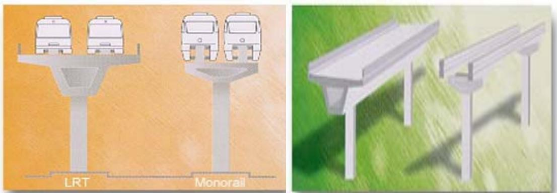
Figure 2.3—Comparison of large-type straddle-monorail with light rail aerials. Source: Monorail Malaysia.
