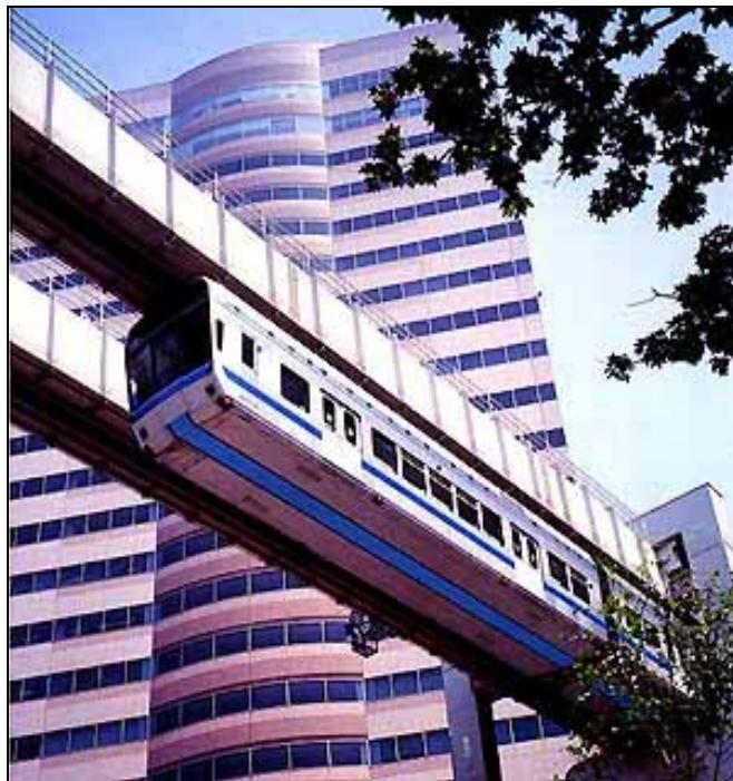
Figure 1.2--Chiba, Japan "Townliner" Suspended Monorail. Source: The Monorail Society
