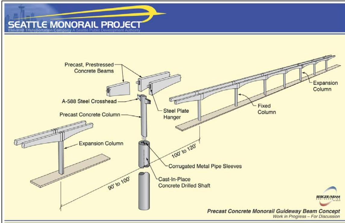
Figure 2.7— The new Seattle Monorail aerial structure may be the best yet. Source: Elevated Transportation Company.
