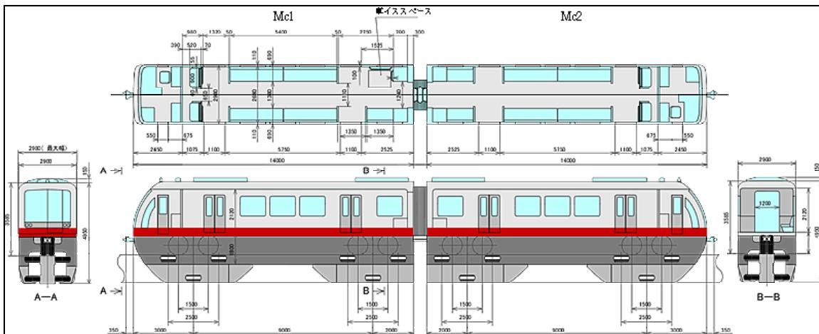
Figure 2.12—Hitachi Series 1000 Monorail for Naha, Okinawa. Hitachi Monorails can be coupled in trains up to 6 cars long. Source: Yui-Rail
